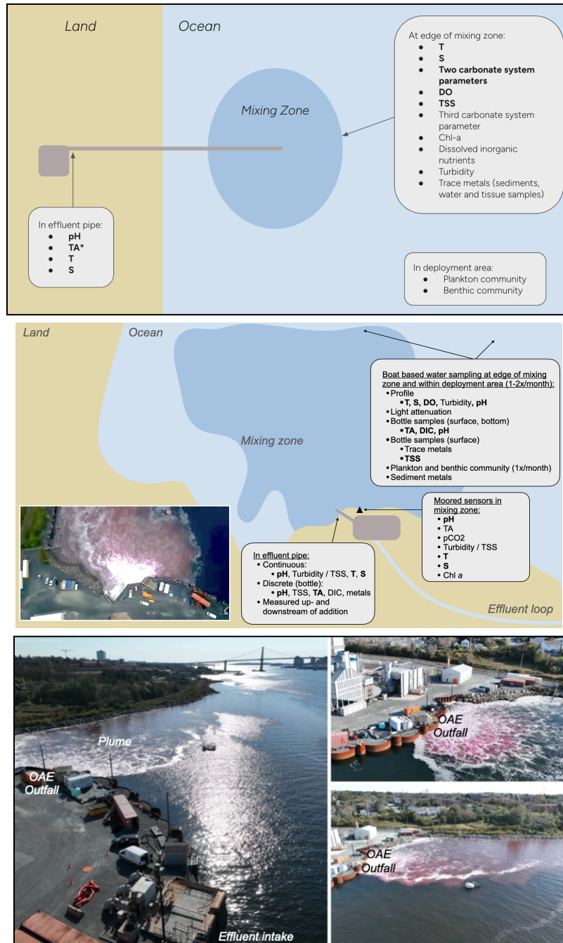
Figure 2.4.2 (TOP) Plan view from Isometric V1.0 OAE protocol Section 10.2 Monitoring Locations. (MIDDLE) Planetary's plan view at Tufts Cove (aerial image inset). Required (bolded) and recommended measurements are listed. (BOTTOM) Zoomed-out images showing the time-varying plume location relative to the OAE discharge.
